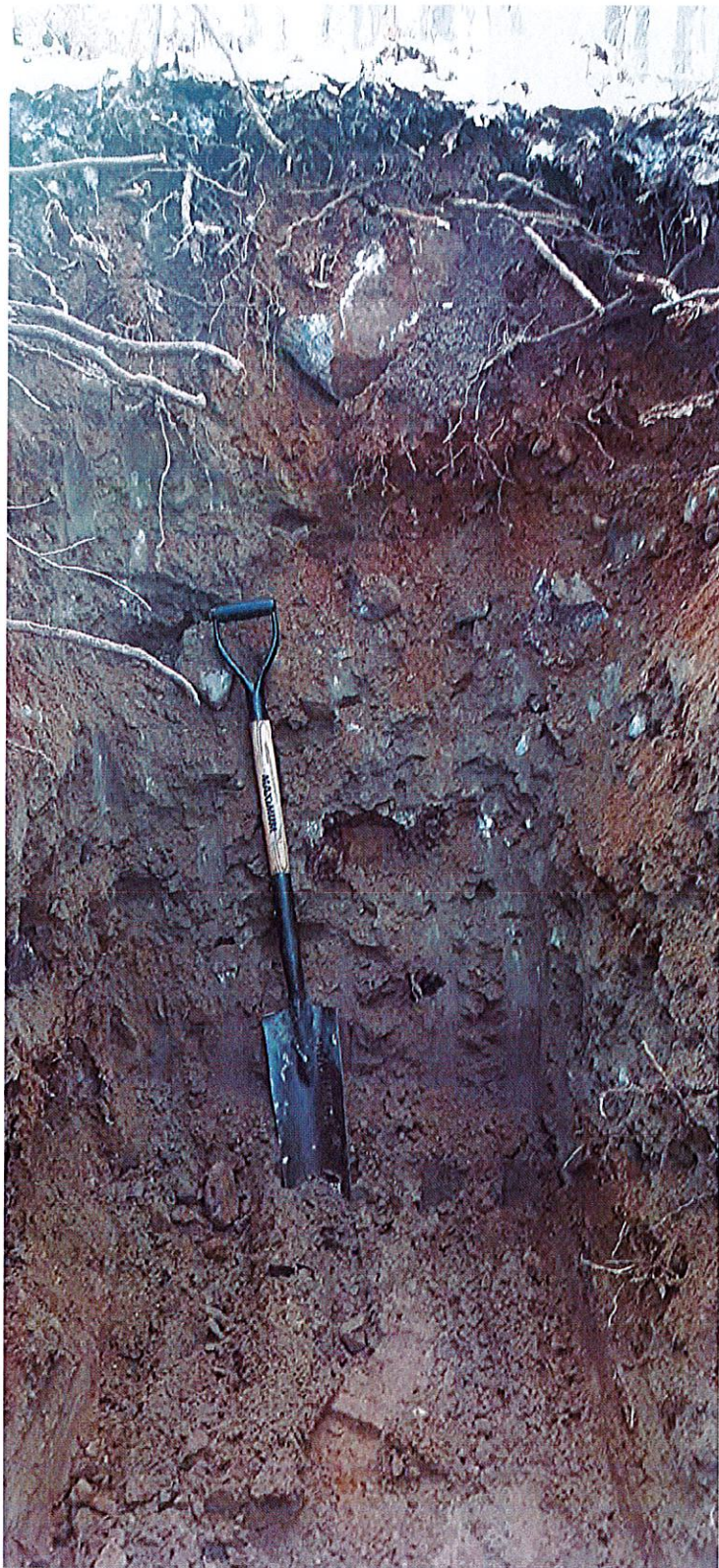
Photo 3 - Test Pit 1 - 2.4 m deep sandy glacial till with no evident groundwater.
