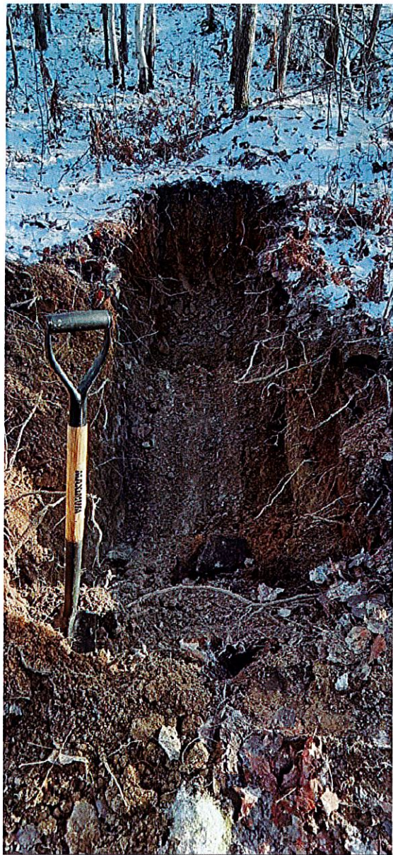
Photo 10 - Test Pit 5 – 0.81 m deep sandy glacial till with no evident groundwater
