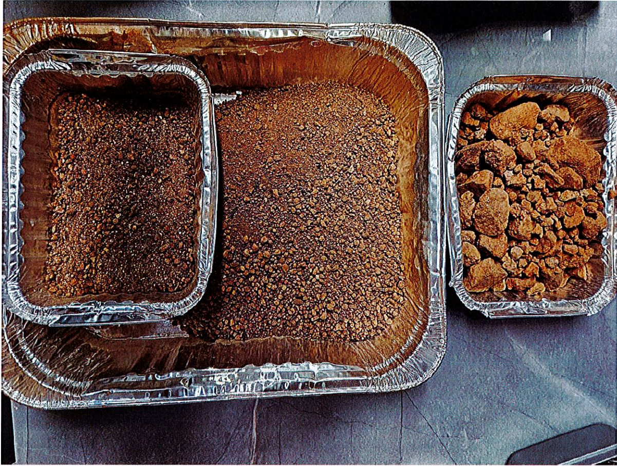
Photo 14 - Sample from Test Pit 3 - 38.5% gravel, 45.6% sand, 16.0% fines
