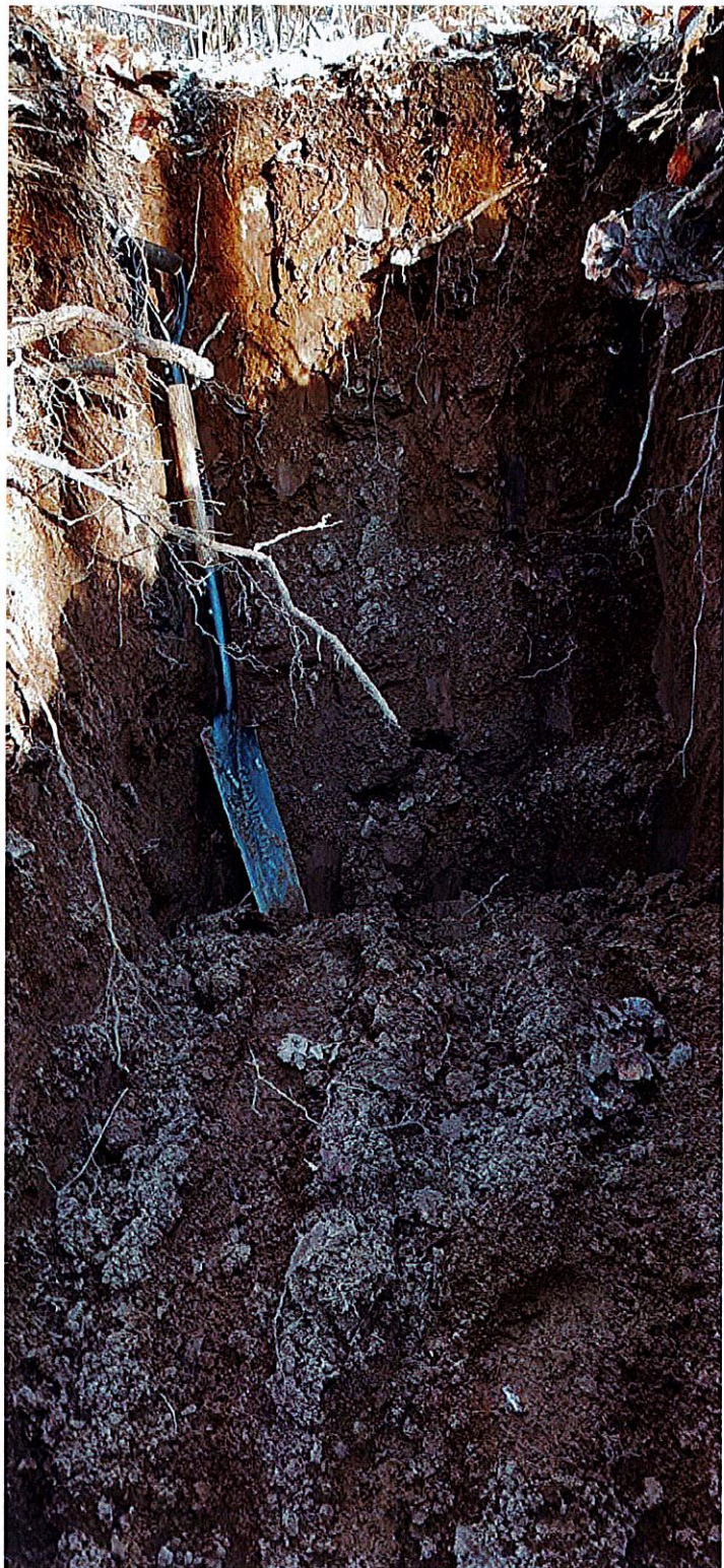
Photot 5 - Test Pit 3 – 1.11 m deep sandy glacial till with no evident groundwater
