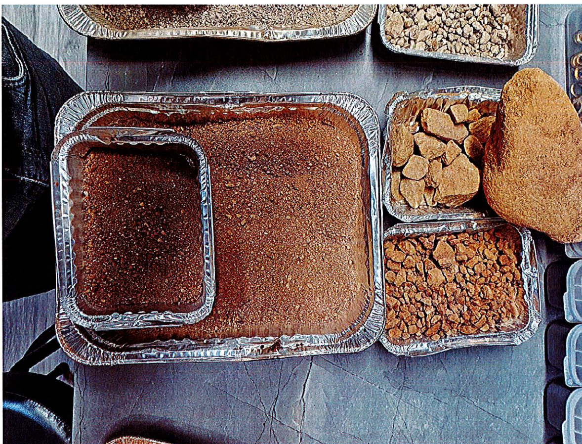
Photo 13 - Sample from Test Pit 1 – 43.7% gravel, 53.8% sand, 2.5% fines.
