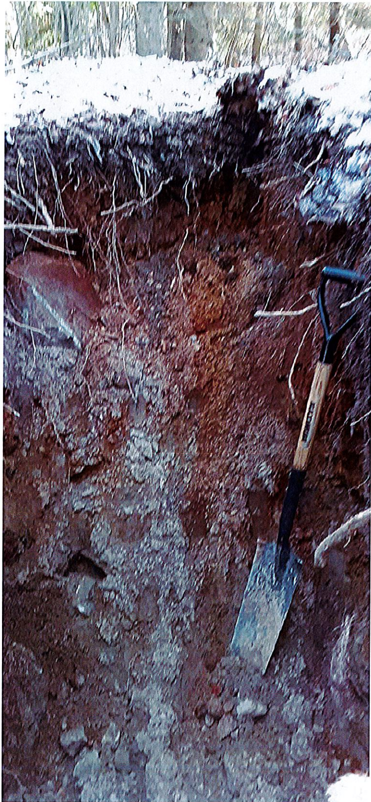
Photo 8- Test Pit 4 - 0.78 m deep sandy glacial till - no evident groundwater.
