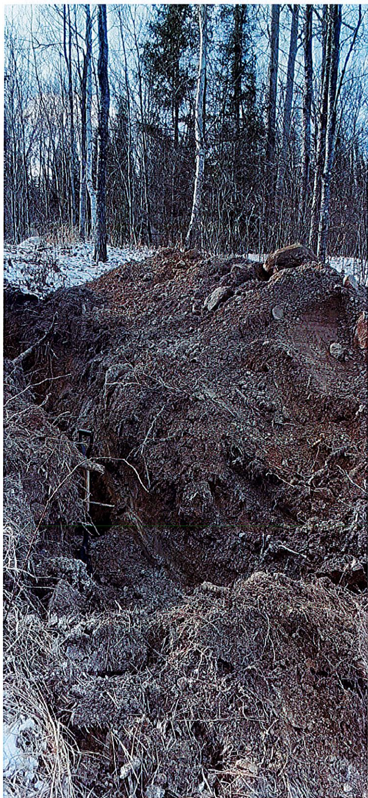
Photo 12 - Test Pit 6 - 1.8 m deep varved silt and clay overlying sandy glacial till
