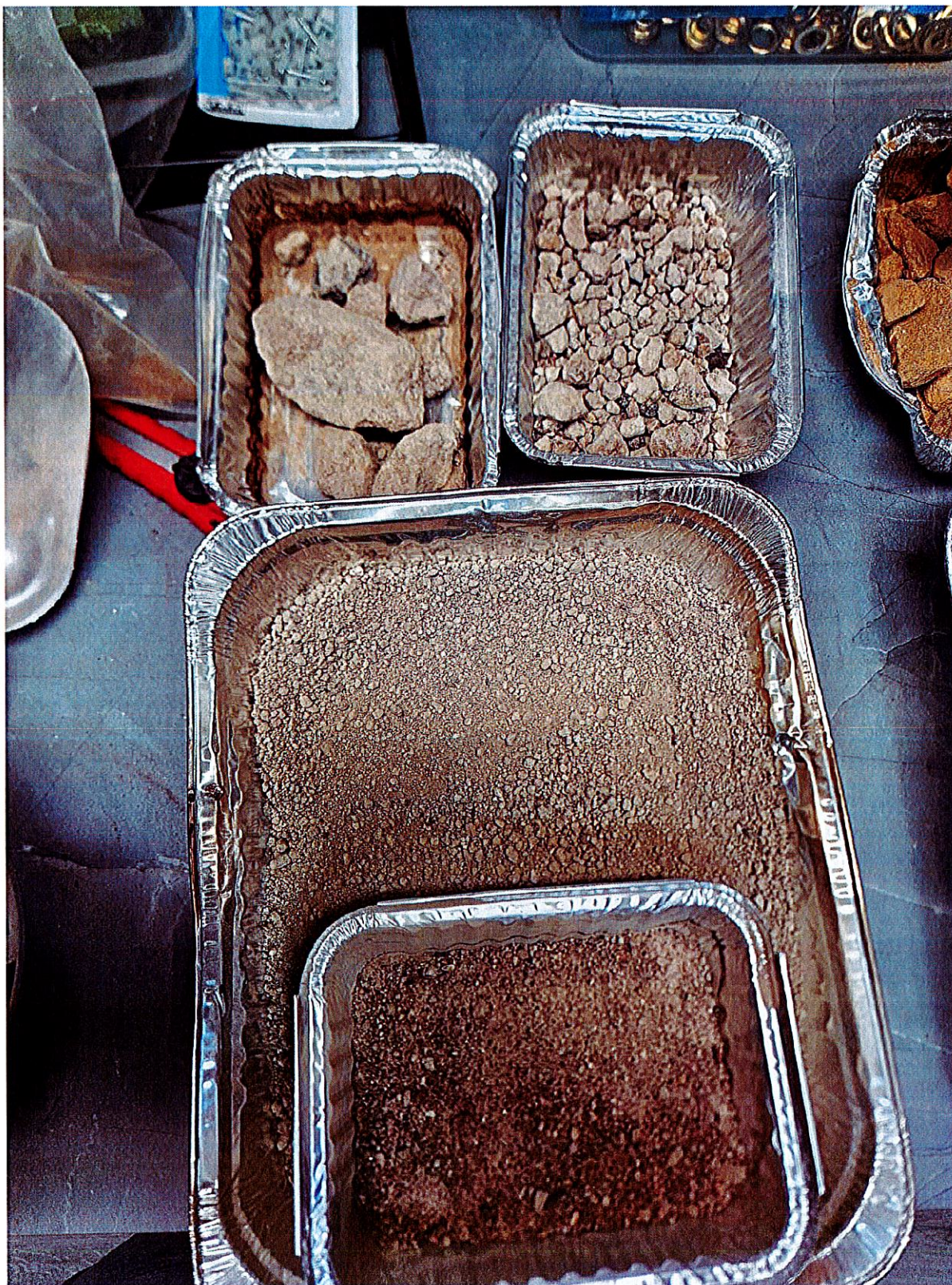
Photo 16 - Sample from Test Pit 5 – 23.2 % gravel, 51.3% sand, 25.5% fines
